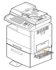
**3** Pull the jammed paper out, in the direction shown, pulling gently and slowly in order to avoid tearing the paper.
